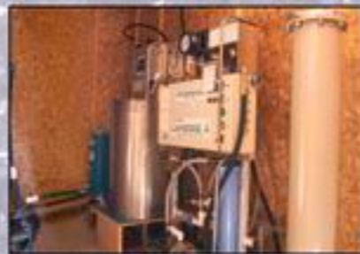
6. The sap is concentrated from 2% to 6% sugar content in a REVERSE OSMOSIS machine
